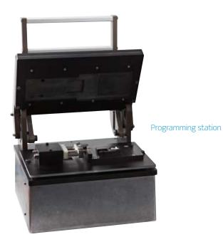
FlexStand Medico typically measures the power consumption of the device, activates inputs, measures outputs and simulates probes needed to make the device run. Mechanical buttons, actuators and connectors can be activated and tested by using a special made fixture. The same goes for optical testing for display control, LED control and dimensional measurements.
