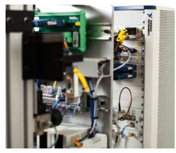
PXI system: RF instrument, Power Supply, Slot-O computer, digital I/O, analog I/O, RS232, USB and Ethernet.
