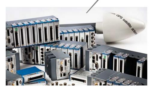
Data capture can be synchronized with GPS for high accuracy.
